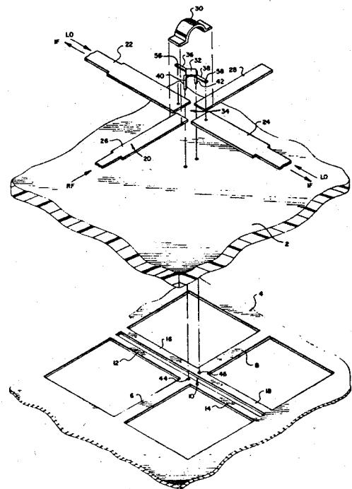
**Symmetric Microwave Mixer with Coplanar Diode Connection**
